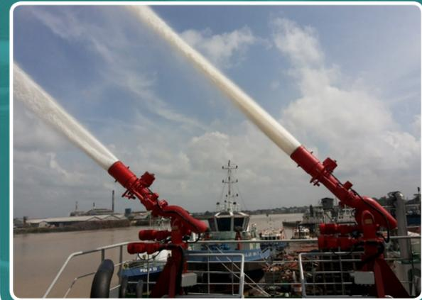
**Geared Monitors:** these allow accurate aiming through the use of a geared system controlled by hand-wheels that overcome the forces that make operation of hand monitors difficult at higher pressures.
