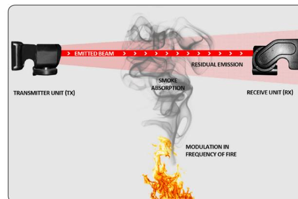
and, in place of the single OBD detector, uses a digital camera type imaging sensor. This technology features high tolerance to vibration and structural movement and gives improved differentiation between smoke and environmental factors like dust and insects. One imaging device can support many emitters making it an efficient means of detection in complex 3-dimensional environments like building atria and theatres.
